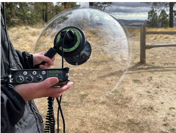
FIGURE 23 Parabolic microphone and field audio recorder used at Kamiak Butte
