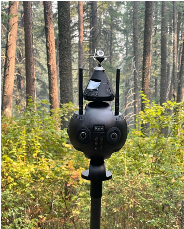
FIGURE 5 Insta360 Pro 2, 360° camera on carbon fiber 3-section tripod
