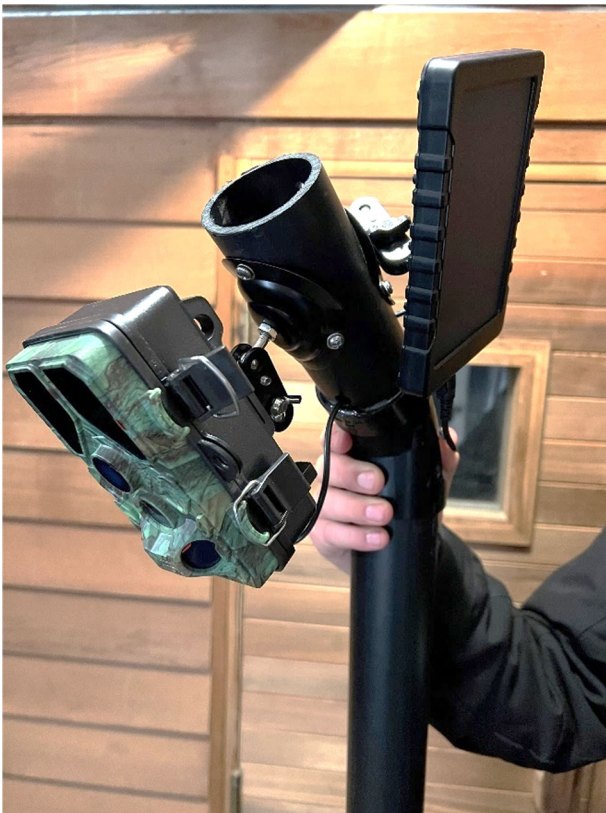
FIGURE 9 CamPark Wi-Fi camera with solar panel apparatus designed for elevated bird nest video capture
