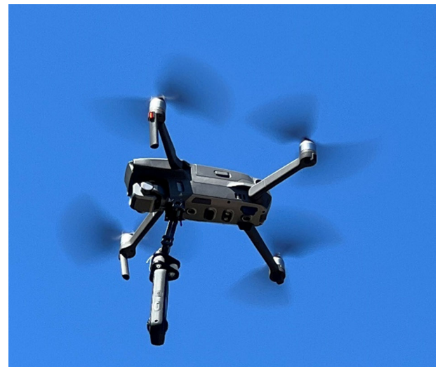
FIGURE 12 DJI Mavic 2 drone vehicle with Insta360 ONE X2 360° camera
